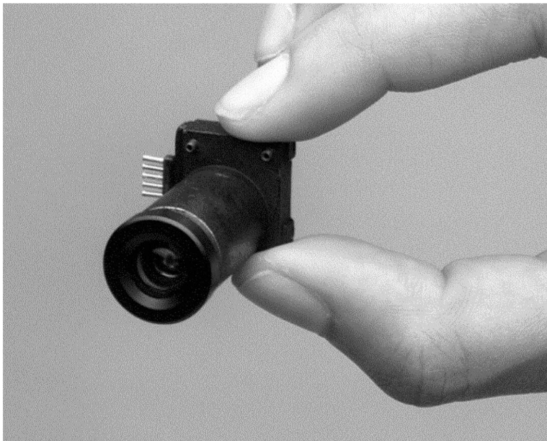
Fig. 11. The JPL single-chip camera with a 512 \times 512 pixel focal plane array. The camera has complete on-chip control and analog to digital conversion circuitry.
